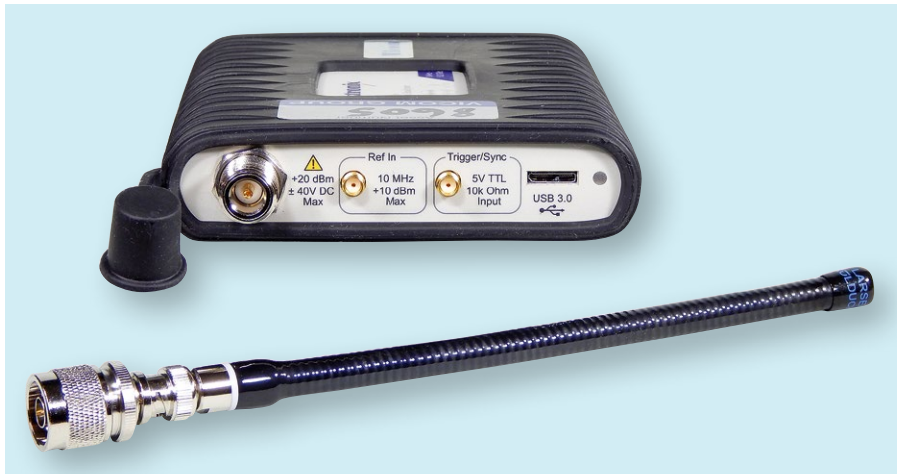
Because it's fully controlled by the SignalVu-PC software, the RSA306 has only four sockets on its front panel. These are (L to R): the main RF input, an input for an optional external 10MHz frequency reference, an external trigger input and the USB 3.0 socket used to connect it to the PC. Also shown here is the helical whip antenna and N-type/BNC adaptor.
